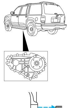
3. Add only enough fluid through the filler opening so that the fluid level is at the bottom of the opening.
